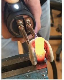
Induction soldering of copper tubes with silver solder.
