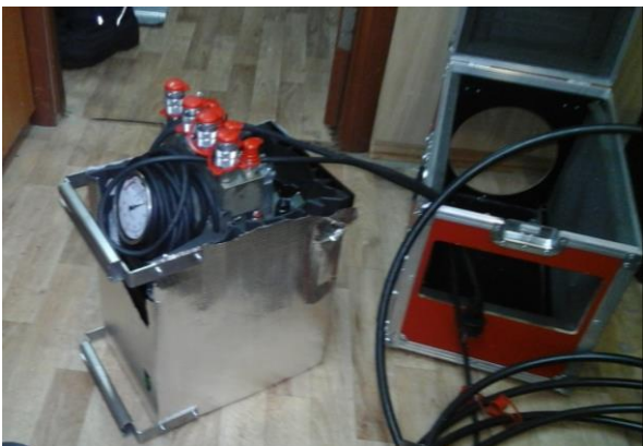
Figure 5: alkitronic Nova pump with additional insulation box
